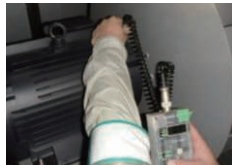
Bearing vibration measurement
